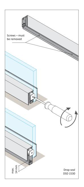
Adjust the drop seal after installation of the door leaf in the door frame.
