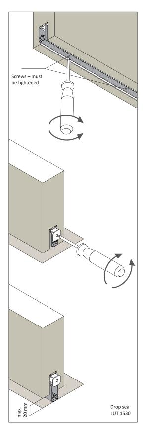
Adjust the drop seal after installation of the door leaf in the door frame.
